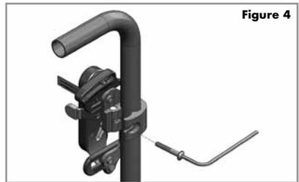
5. Repeat steps 2 through 4 for the opposite clamp ensuring the clamp is set at the same height as the opposite side previously installed. Attach the back shell by guiding the bottom attachment pins into the lower receiver slots and then pushing the top attachment pins into the latch mechanism. Be sure both latch buttons pop back, and tug the back shell forward to verify that it is secure.
